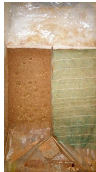
Fig. 5 Industry (M/s Geosol Associates) Sponsored Research Project on Embankment erosion control (Rainfall simulator and embankment model without and with protection)
