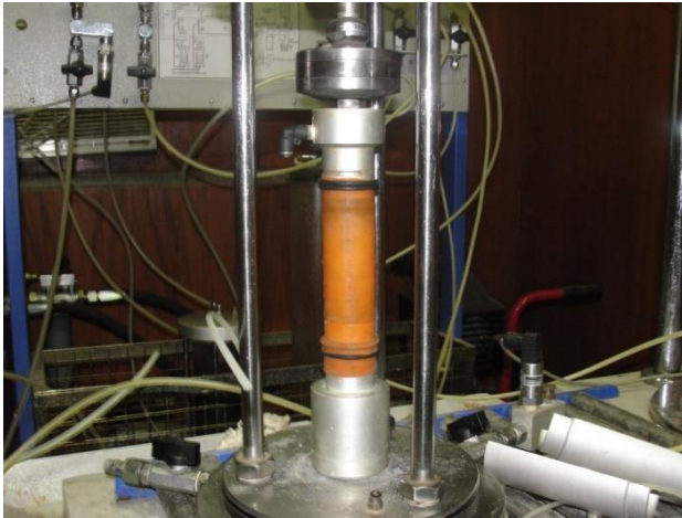
Fig. 1 Specimen before and after the tests in a PC Controlled Cyclic Tri-axial facility
