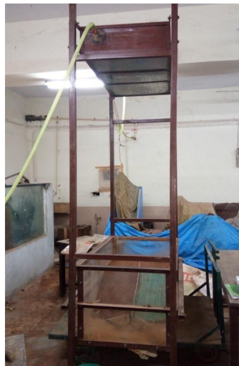
Fig. 5 Industry (M/s Geosol Associates) Sponsored Research Project on Embankment erosion control (Rainfall simulator and embankment model without and with protection)
