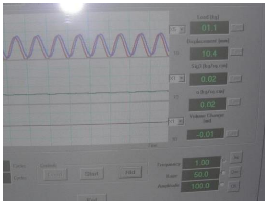
Fig. 4 Cyclic Load Tests on compacted pond ash test bed
