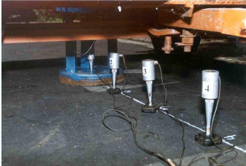
**Falling Weight Deflectometer (FWD) – A Low cost model**
