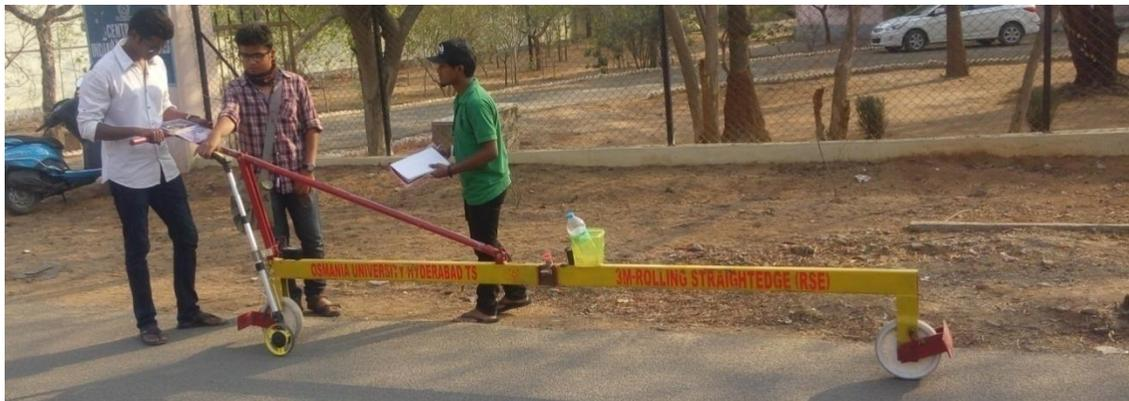
Measurement of Unevenness of Roads in Osmania University by Using **ELECTRONIC 3-M ROLLING STRAIGHT EDGE (ERSE)**
