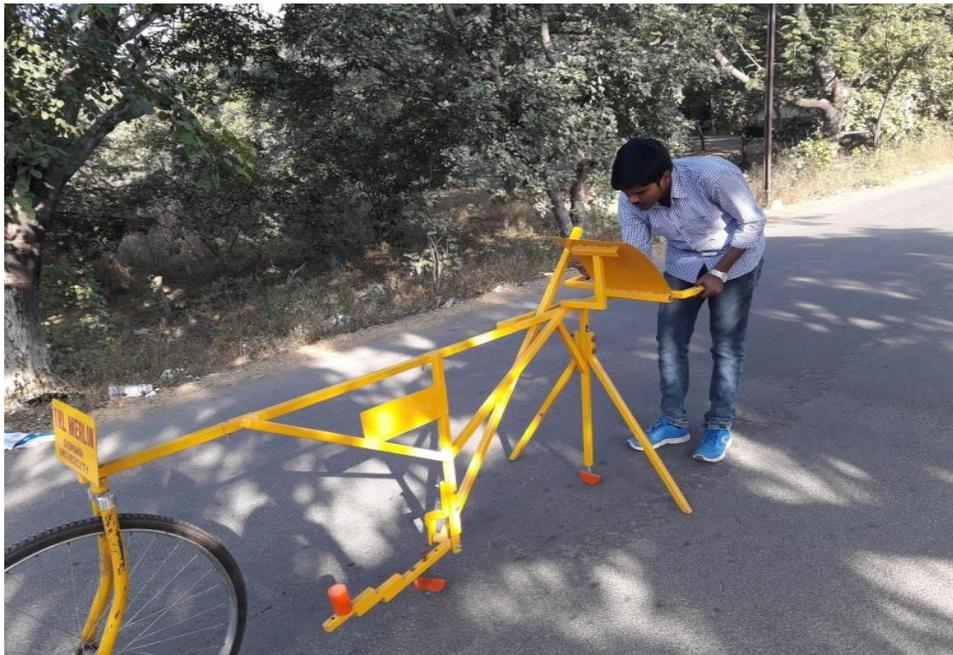
**Machine Evaluating Roughness using Low-cost Instrumentation (MERLIN)**
