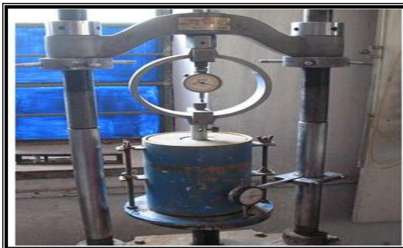
TYPICAL COMPRESSION TESTING MACHINE (CTM) USED FOR CBR / TRIAXIAL COMPRESSION TESTS
