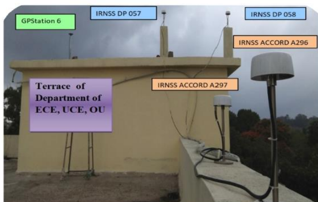
GNSS Antenna's Setup for Real-time Data Acquisition(AGRL)
