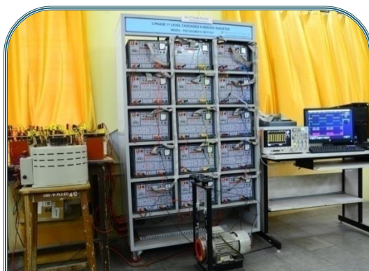
Three Phase Eleven – Level Cascaded H-Bridge Inverter
