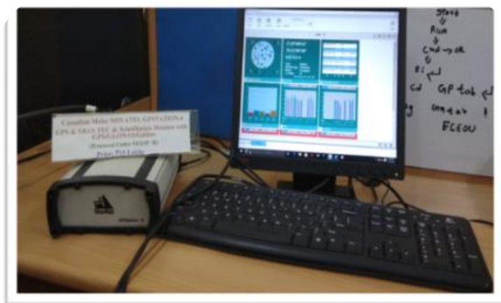
Novatel GPStation-6 GPS/Glonass/Galileo/Beidou/QZSS Triple frequency Satellite Navigation Receiver
