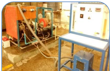
Multi cylinder 4 stroke petrol engine test rig
