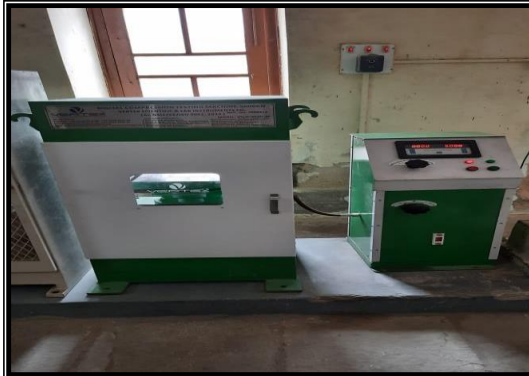
Compression Testing Machine Capacity: 5000 KN
