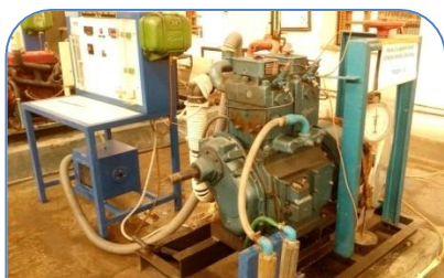
Twin cylinder 4 stroke diesel engine test rig
