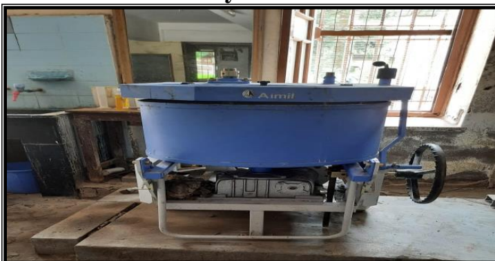
Concrete Pan Mixer, Capacity: 40 L,
