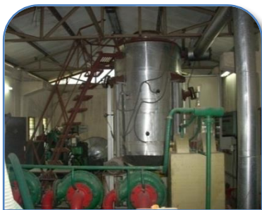
Advanced Biomass Downdraft Gasifier
