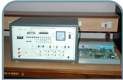
IPM Power Module with DSP Controller
