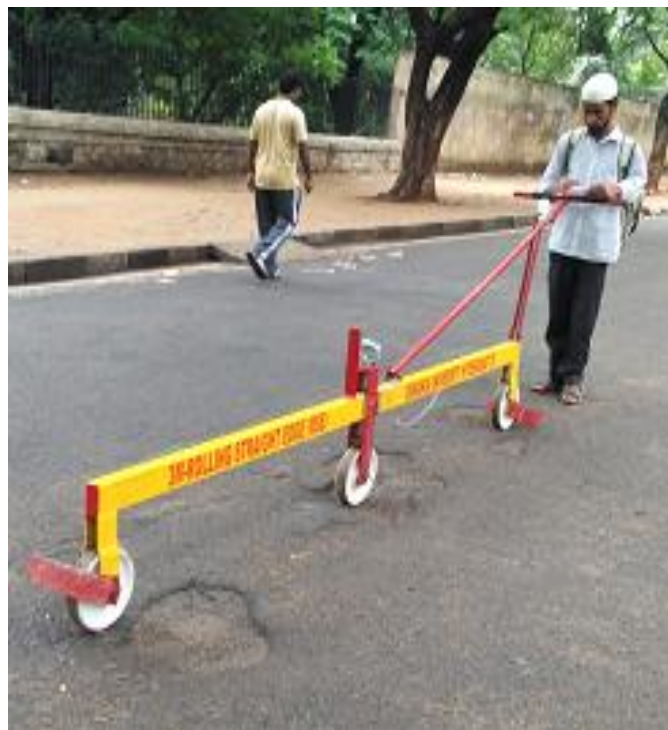
3-M Rolling Straight Edge- A Basic Model
