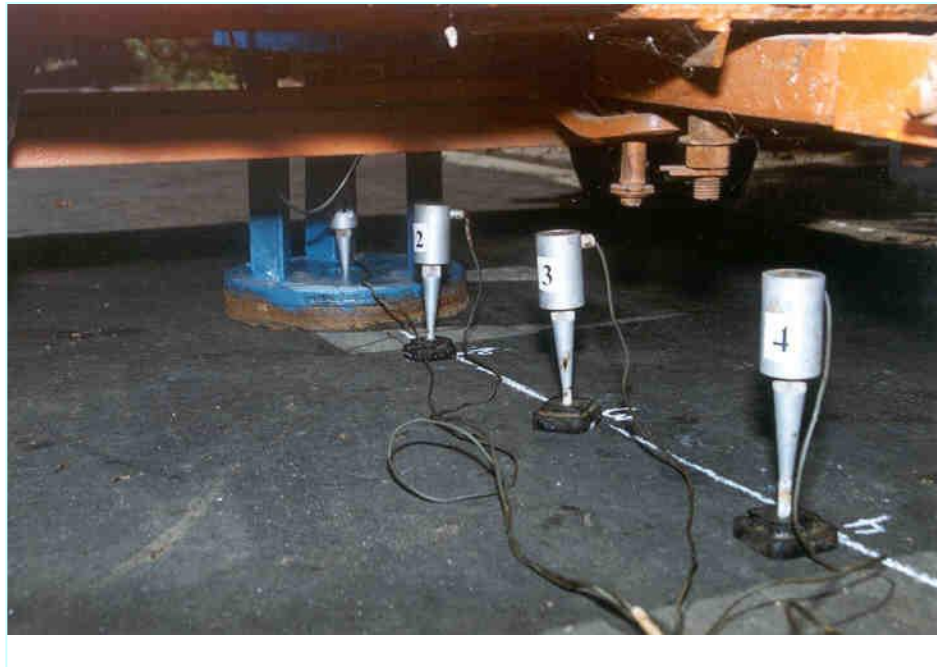
Falling Weight Deflectometer (FWD) – A Basic Model
