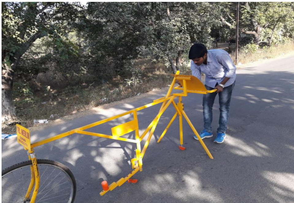
Machine Evaluating Roughness using Low-cost Instrumentation (MERLIN)
