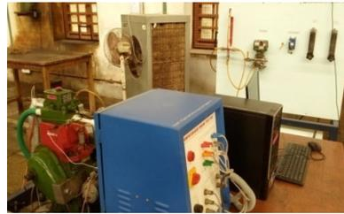
Twin cylinder 4 stroke diesel engine test rig
