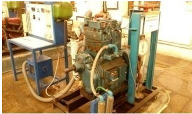
Variable Compression Engine test rig
