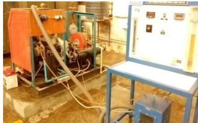
Multi cylinder 4 stroke petrol engine test rig
