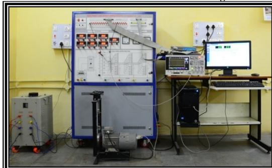
**Three Phase Seven-Level Neutral Point Clamped Inverter**
