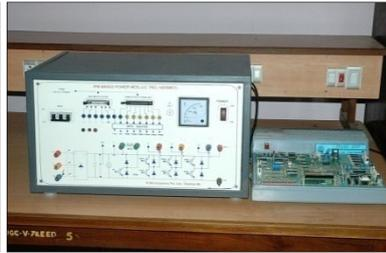
**IPM Power Module with DSP Controller**
