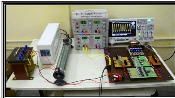
**Cascaded Seven- Level Asymmetrical Inverter with Reduced Switches**
