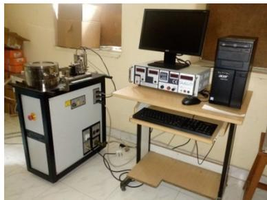
Pin on Disk tester equipment in Metrology Lab
