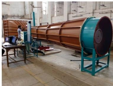
Subsonic wind tunnel testing in Thermal Lab
